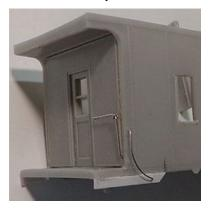
9. Now we need to drill a hole in the roof for the smoke stack. The smoke stack base is 2.33 mm. After drilling the hole, we test fit the smoke stack.
